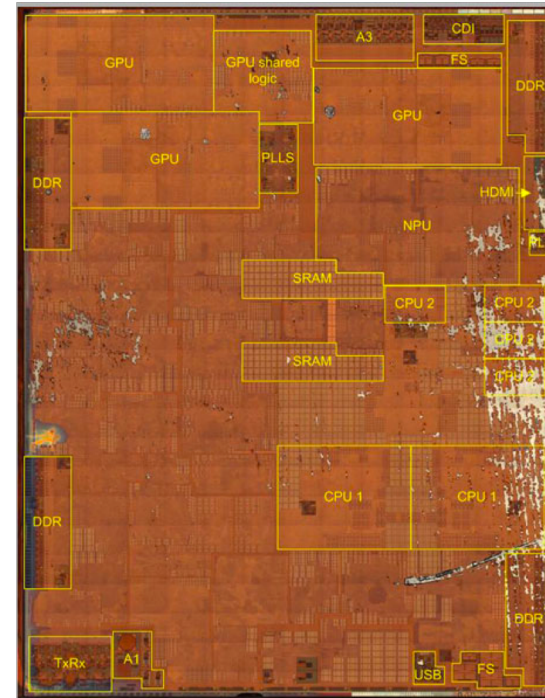
Apple A11 Bionic* Two "high performance" 64 bit ARM CPU cores Four "low performance" ARM CPU cores Three "core" Apple-designed GPU Image processor Neural Engine for DNN acceleration Motion processor
