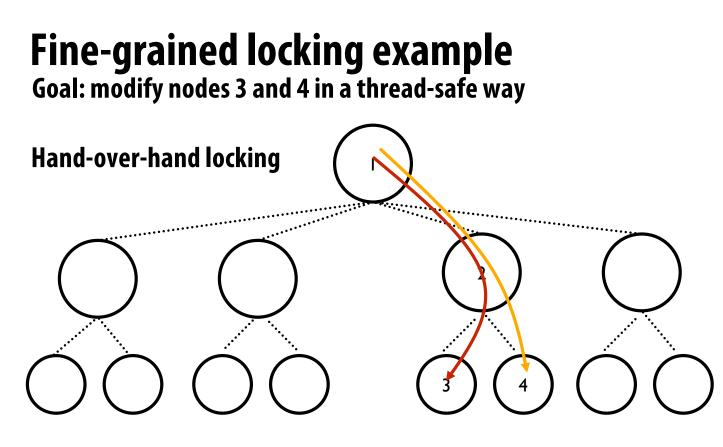
Locking can prevent concurrency (here: locks on node 1 and 2 during update to node 3 could delay update to 4)
