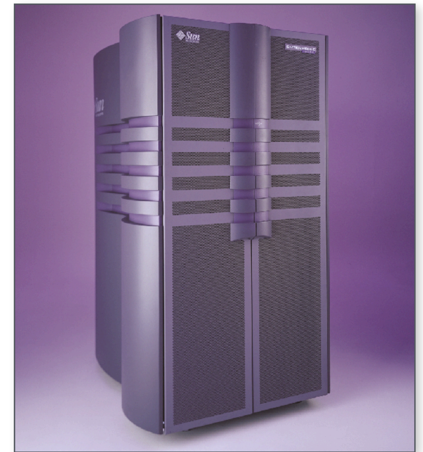
Sun Enterprise 10000 (circa 1997) 64 UltraSPARC-II processors
