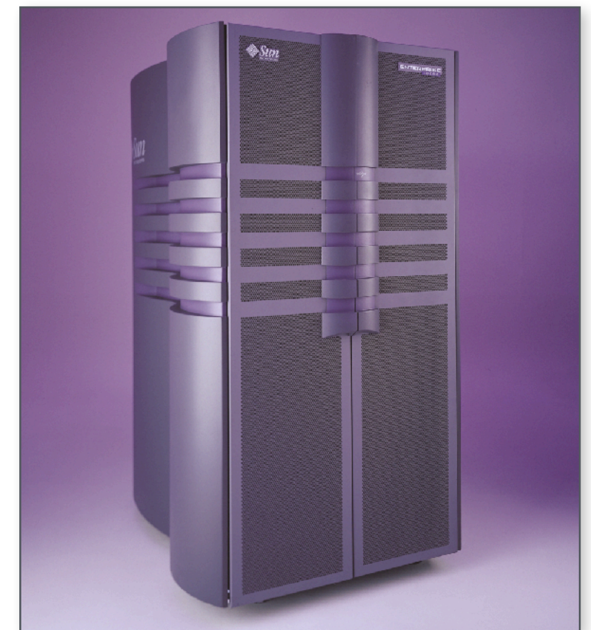
Sun Enterprise 10000 (circa 1997) 64 UltraSPARC-II processors
