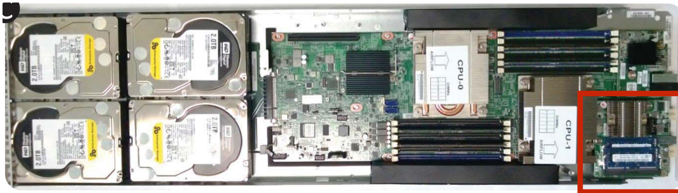
1U server (Dual socket CPU + FPGA connected via PCIe bus)
